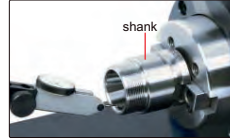
measure radial runout of shank
